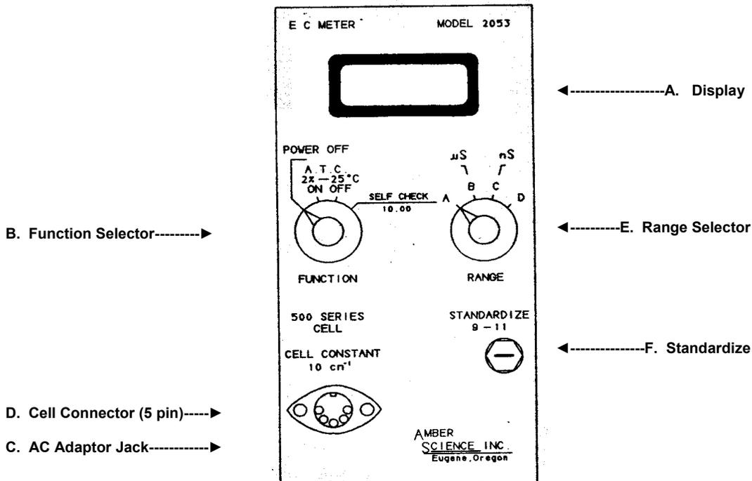
**(A) Display:** 3 ½ Digit LCD with floating decimal and “Lo Batt” (low battery) indicator.
