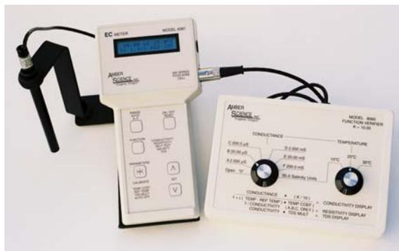
Model 4081 shown with Dip Cell, Lab Stand and Function Verifier
